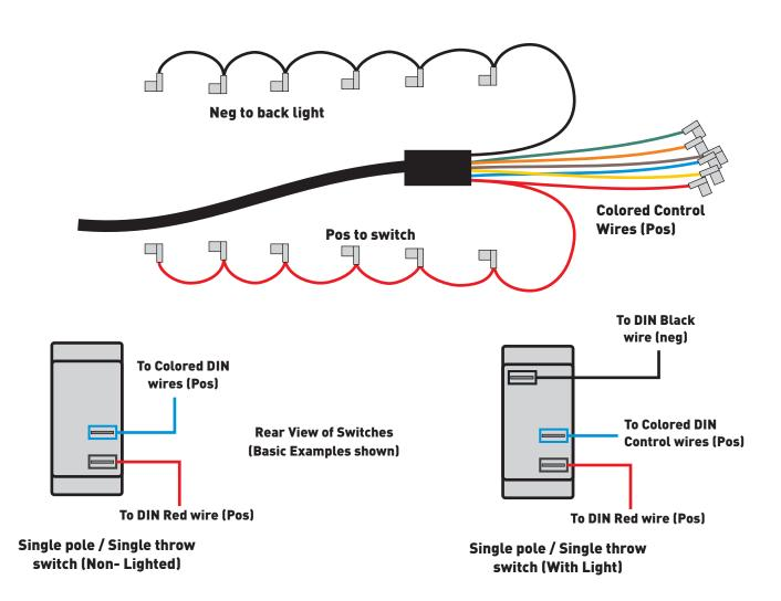
Wiring the DIN on a 6 Shooter or 4 Plus to a switch requires the connections as shown above.
